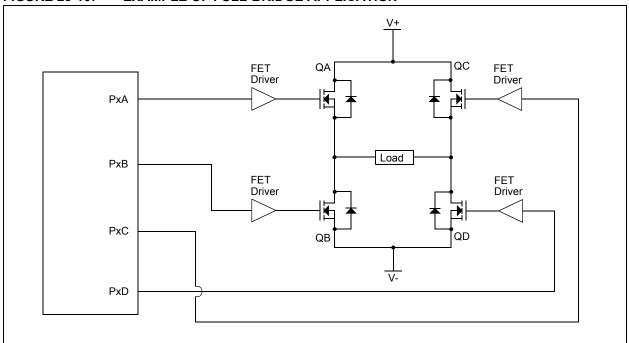
FIGURE 23-11: EXAMPLE OF FULL-BRIDGE PWM OUTPUT
