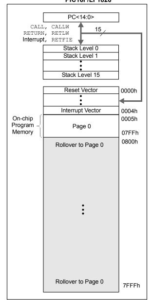
FIGURE 3-2: PROGRAM MEMORY MAP AND STACK FOR PIC16F/LF1827
