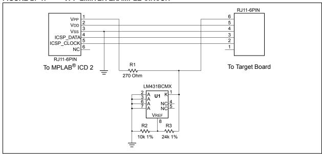
**Note:** The ICD 2 produces a VPP voltage greater than the maximum VPP specification of the PIC16F/LF1826/27.
