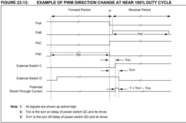
**EXAMPLE OF PWM DIRECTION CHANGE AT NEAR 100% DUTY CYCLE**
