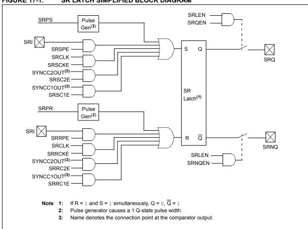
FIGURE 17-1: SR LATCH SIMPLIFIED BLOCK DIAGRAM
