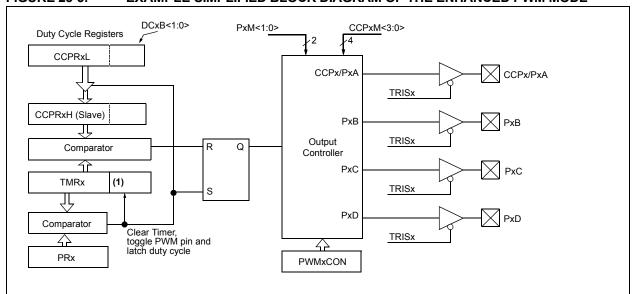
Note 1: The 8-bit timer TMRx register is concatenated with the 2-bit internal Q clock, or 2 bits of the prescaler to create the 10-bit time base.
