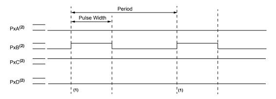
Note 1: At this time, the TMRx register is equal to the PRx register.
