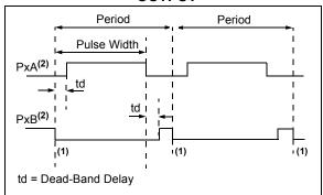
**Note 1:** At this time, the TMRx register is equal to the PRx register.
