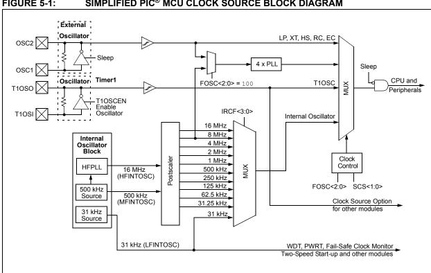
FIGURE 5-1: SIMPLIFIED PIC® MCU CLOCK SOURCE BLOCK DIAGRAM
